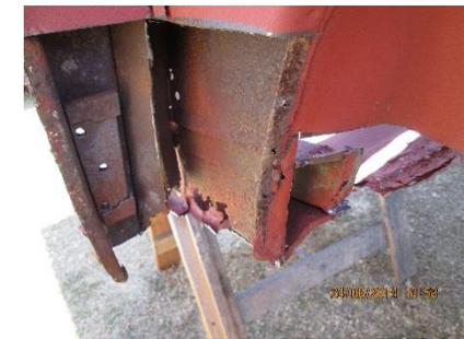
The extent of rust can be seen on the lower panels. The two floor boards will also have to be replaced.
