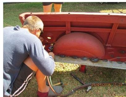
The Cab has been completed. All rusted panels replaced, coat of self-edge primer applied. Underneath and inside sprayed with stone chip, and a coat of 2K Satin black. Next was the load body that was sand blasted, rusted panels replaced. Body and panels are ready for the spray painters. Then the rewarding parts starts, assembling the Van.
